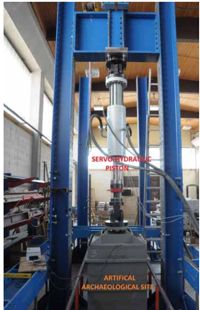
Figure 3. Servo-hydraulic piston and metal box with the artificial archaeological site.
