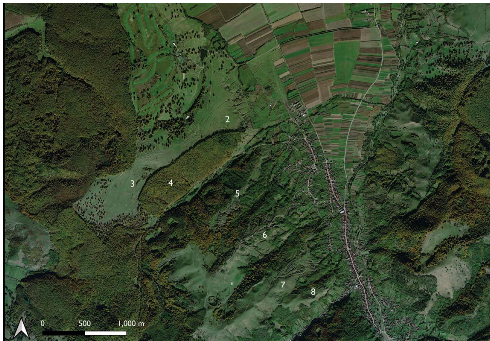
Fig. 8. Satellite view of the workings at Pianul de Sus, Romania. 1: Area of small pits to the east of the modern golf course. 2: Plateau incised by channels which develop into deeper hush-gullies at the eastern edge. 3: Hushing tank with channel discharging into 4, a now wooded hush-gully. 5, 6, 7, 8: Ridges whose flanks are dissected by ground-sluicing channels. The village of Pianul de Sus extends along the road to the right of the centre of the image (satellite image: Bing Virtual Earth, with annotations by A. Wilson, 2023).
